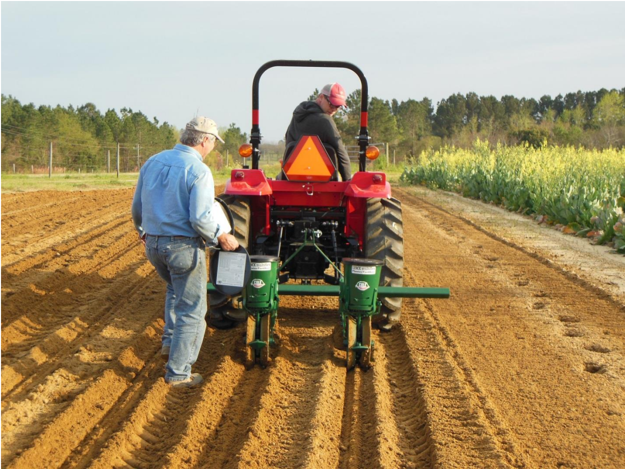
Frank's Designs for Peanuts, LLC - 2 Cole 12MX planters mounted on a toolbar during testing at the Blackshank experiment farm in Tifton, GA, prior to shipment to Haiti
