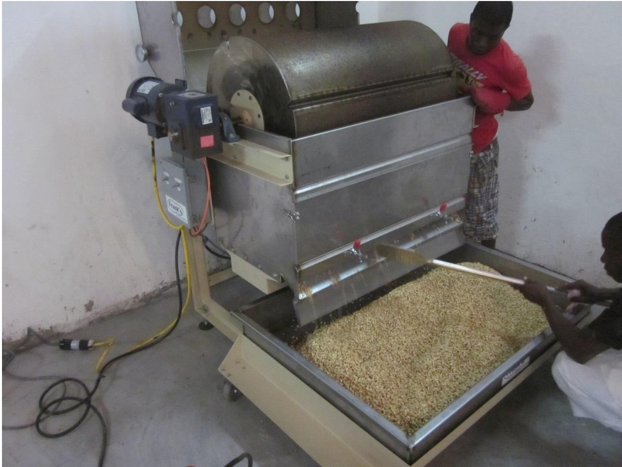
Frank's Designs for Peanuts, LLC – Finish roaster being used at the Project Peanut Butter facility in Sierra Leone, Africa
