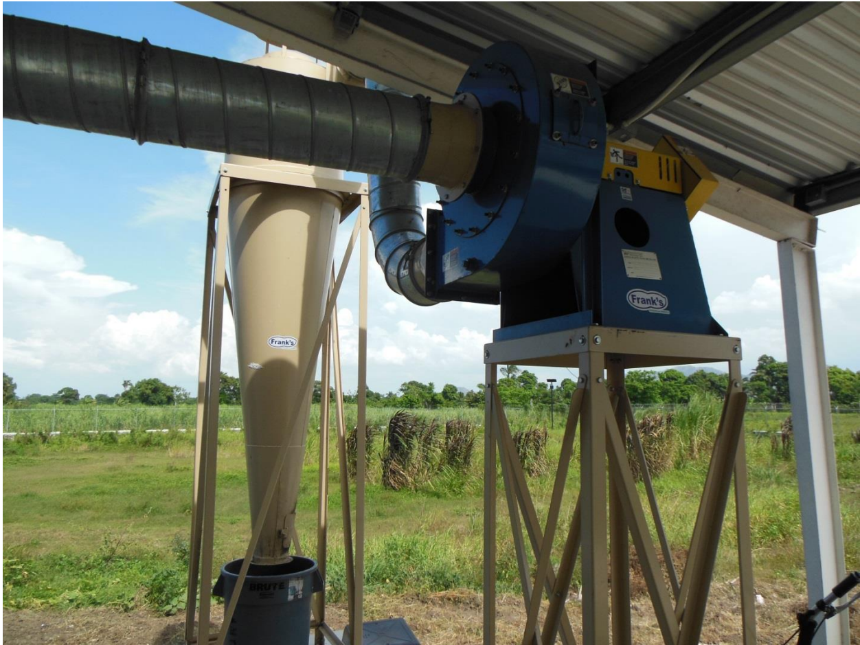
Frank's Designs for Peanuts, LLC – Dust collector & fan @ Meds & Foods for Kids Haiti
