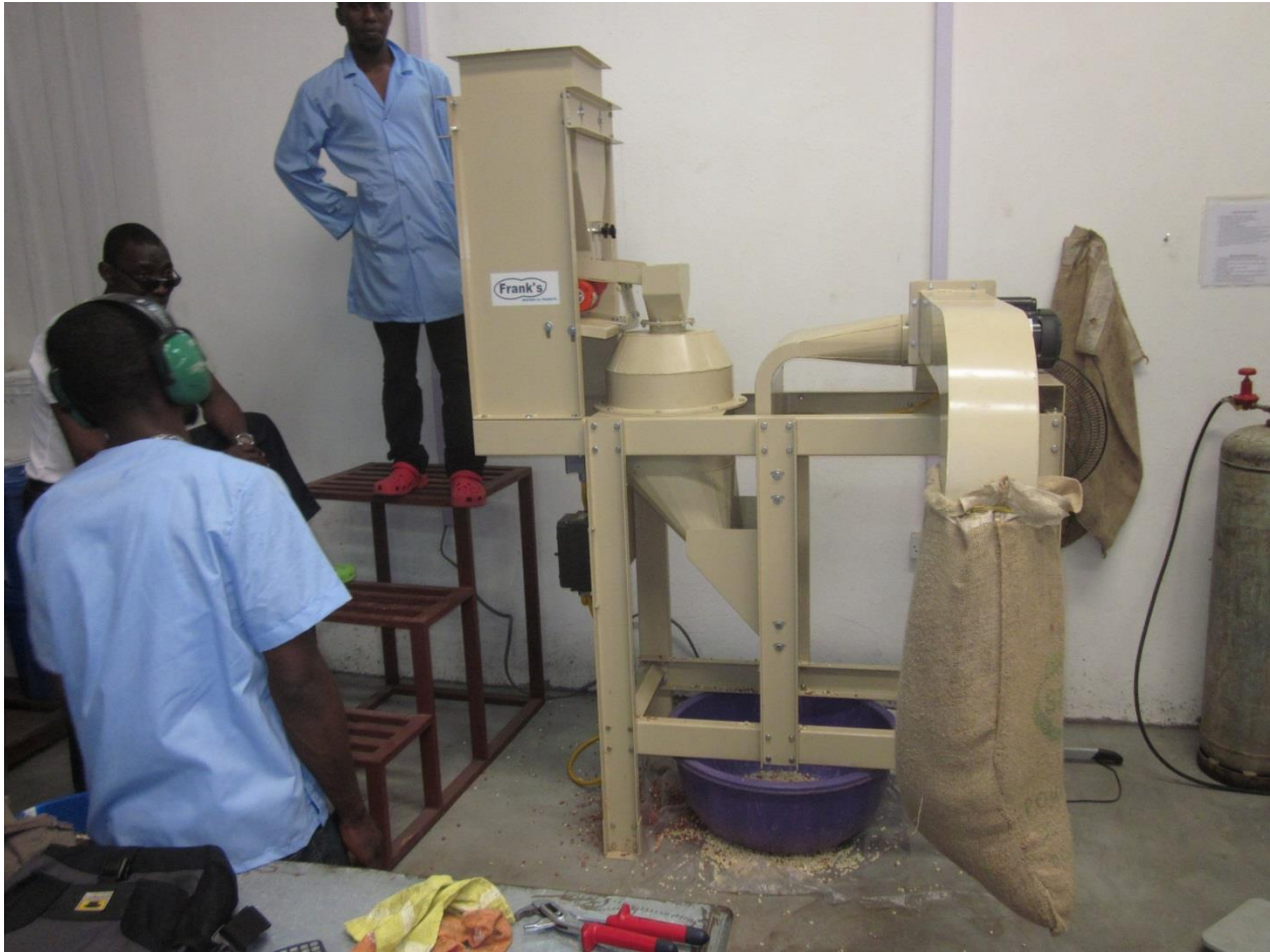
Frank's Designs for Peanuts, LLC – Splitter/blancher in use at the Project Peanut Butter facility in Sierra Leone, Africa
